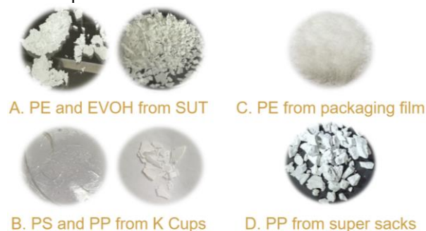
Figure 3. Pure plastic after STRAP processing of waste: A. PE (left) and EVOH (right) from single use pharmaceutical waste [9], B. PS (left) and PP (right) from single use Keurig cups C. PE from multilayer films [8], D. PP from super sack fabric
